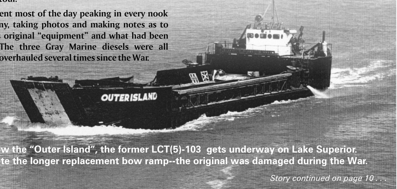
Now the "Outer Island", the former LCT(5)-103 gets underway on Lake Superior. Note the longer replacement bow ramp--the original was damaged during the War.
