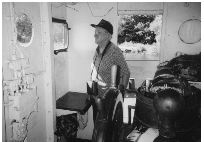
Inside the pilot house of the Outer Island. Larger portholes and a new binnacle have been added since the War.
